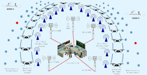
Monitoring for Unauthorized Access with Interdiction - A motion sensor is alerted to movement at strategic locations. This triggers an investigation by aiming a camera at the particular point. If selected behavior is seen a drone will be dispatched to fly above the area to monitor and count the people involved and take photos. Unmanned afloat systems (WAM-V) perform support roles as needed in the water.
